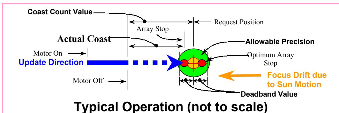
A comparison between the sun angle and the array position is performed by converting the sun angle to array position coordinates (counts) using an equation involving **Gear Ratio**, defined here as **Counts per Radian** (radian = angular arc / radius of arc) then adding in a **Reference Offset** (in counts also) from a fixed zero point established by a **Reference Point (RP)** indicating where in the mechanical range of motion a particular count number occurs such that:
