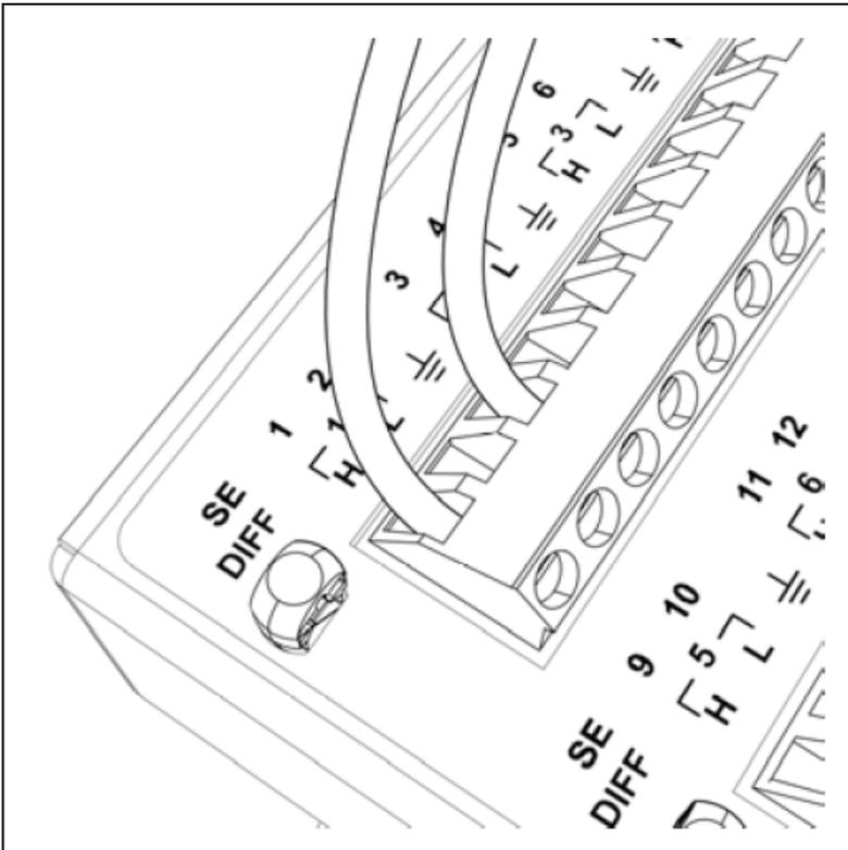
A typical single-ended input connection – this one to S.E. #1 – there will usually also be a braided shield wire that is connected to the ground terminal ( $\perp$ ) next to it along with the standard ground reference wire... all ground wires going into a single grounding terminal should be twisted together before inserting into the terminal block to reduce the possibility of 'whiskers'.
