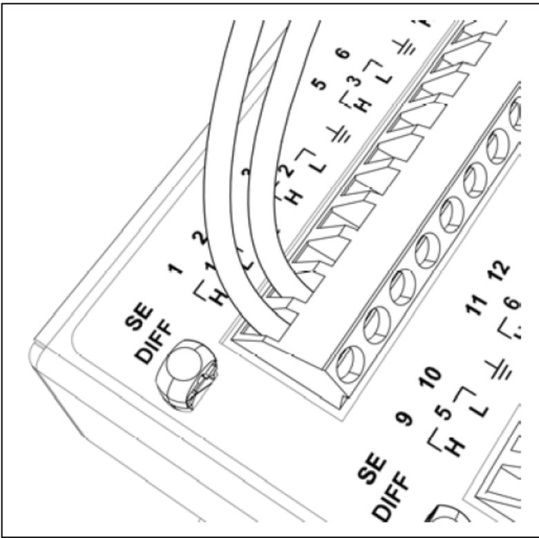
A typical differential input connection – to the left, Diff. #1 – and below in the picture, Diff. #7 – there will usually also be a braided shield wire that is connected to the ground terminal ( $\perp$ ) next to it.
