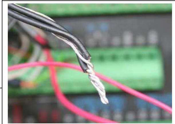
Five of the six weather instruments require 5 VDC power. In each case, except for the rain bucket, the red wire will need to be attached to the +5 V terminal on the datalogger... the unit is shipped with a single red wire already attached to the 5V terminal... this wire and a second wire attached to the two pull-up resistors will be joined with the five power leads of the weather instruments.
