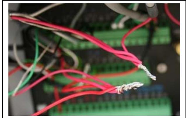
Two pull-up Resistors join the Wind Speed input in P1 and the Rain Bucket input in P2... the other end of the pull-up resistor wire joins the other 5V power leads in the wire nut...
