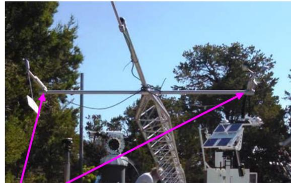
Slide the bases into the sleeves on the crossbar and use the larger of the two hex wrenches in the box to snug down the set screws on both devices.
