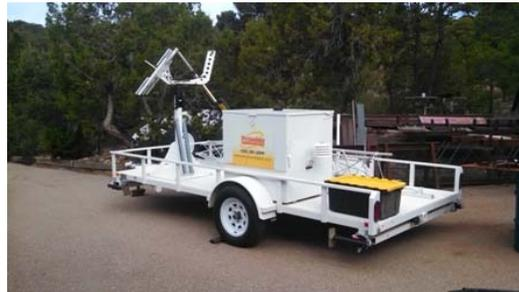
If low-level wind instruments are installed, one mounting strut is folded and clamped for travel. Remove the clamp then lift the tower base to ease it out from under the rail and fold it under to point the opposite direction.
