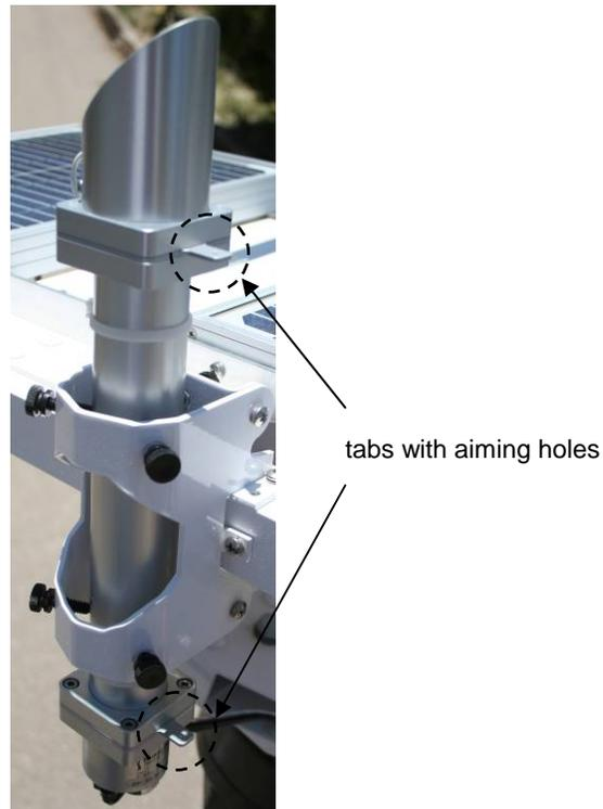
**Note:** Only align the DNI sensor once the Prospector is aimed accurately at the sun. It helps to have bright sunlight to aim the DNI sensor
