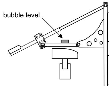
Level the Prospector facing each direction, east, south, and west (east, north, and west in the southern hemisphere). Compare the measurements. It is better to have the level be off by the same amount in each direction than to have it perfectly level in one direction and farther off in another.
