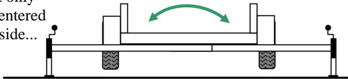
Pull the jack locking pins and rotate jack downward until the spring lock engages...
