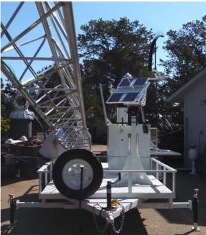
The tracker should be rotated slightly and raised about twenty degrees (joystick up) so that the tower will miss the tracker and the wind vane mounting strut will miss the base of the screwjack.
