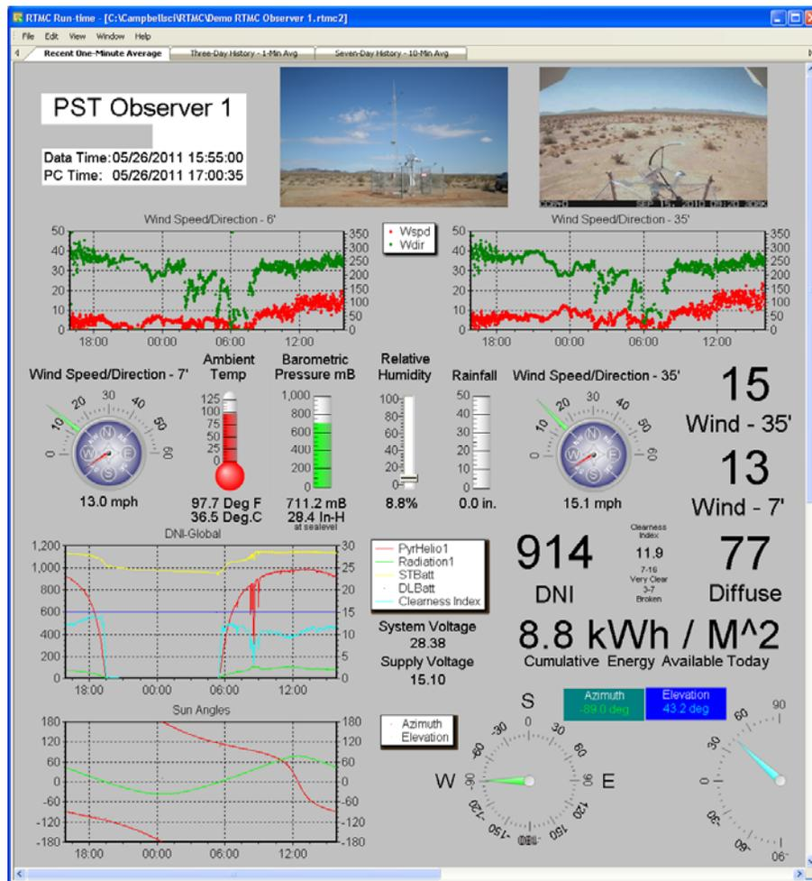
This screen layout is designed for at-a-glance assessment of current and recent solar and weather conditions. Its pictorial GUI presentation of data (meters, dials, slides, etc.) is augmented by digital fields with the actual number and units represented.
