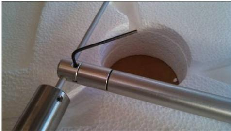
There are two small hex wrenches stuck into the foam inside the wind instrument box. The little one is for attaching the rotors to the masts.
