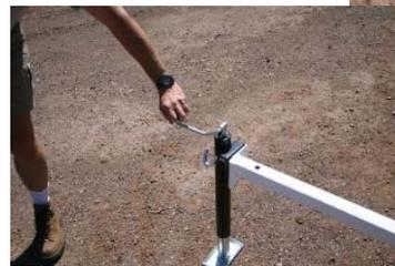
Moving to the forward outriggers, refer to the bubble level mounted on the azimuth deck (Pg. 14) to adjust the forward jacks until the bubble is centered...
