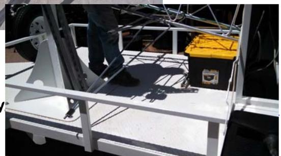
Once unfolded, use the removed clamp and a second one attached loosely to the opposite rail to securely clamp the mounting arm.
