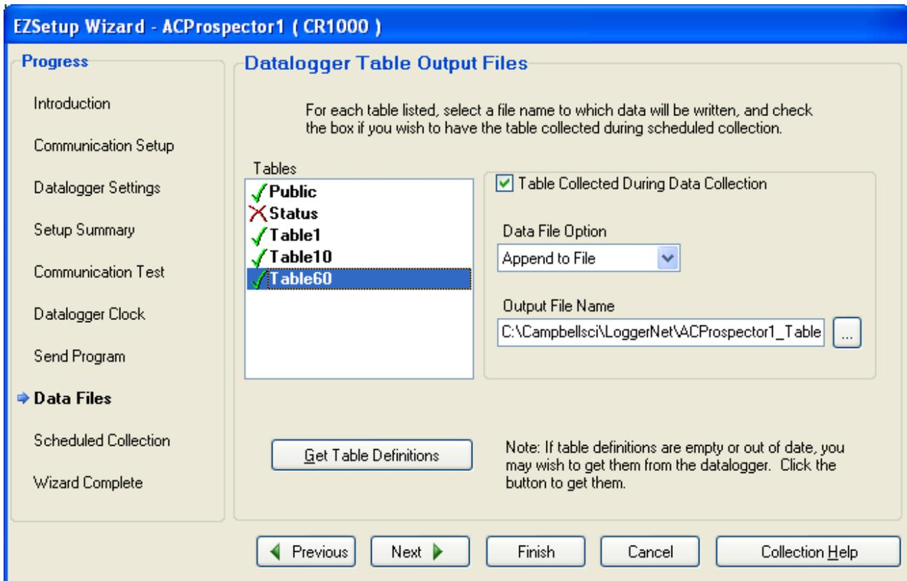
The 'Public' table is actually a type of 'internal common block storage' for the sampled data, computations, status variables and other working variable applications through which tasks are accomplished or controlled in the datalogger program. The green checkmarks correlate with the check box to the right labeled 'Table Collected During Data Collection'.
