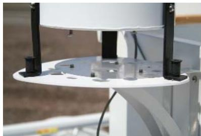
Attach the feet to the mounting plate such that the wire is toward the corner of the storage box...
