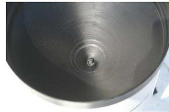
Remove packing material, screens and locate the cable tie inserted in the collection hole...
