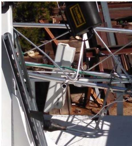
The site camera is mounted on a short rod already attached to the tower base just above the low-level wind instruments which extends out to the right side of the trailer. It should be oriented at a right angle to the tower base rail and with that orientation will offer a reasonable sky shot as well as the Prospector unit itself in the lower left corner of each frame as a monitoring mechanism. Experience indicates the u-bolt must be very firmly tightened to avoid rotation from gravity.
