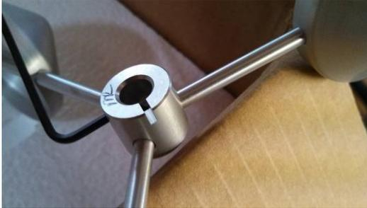
The Met One wind instruments in the large, flat box are stored partially disassembled... each has a registration post on the stem and a matching slot in the rotating heads...
