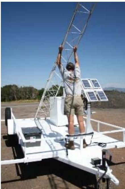
Fully insert the rear tower rail into the mounting flange, aligning the two top holes and insert the locking pin.
