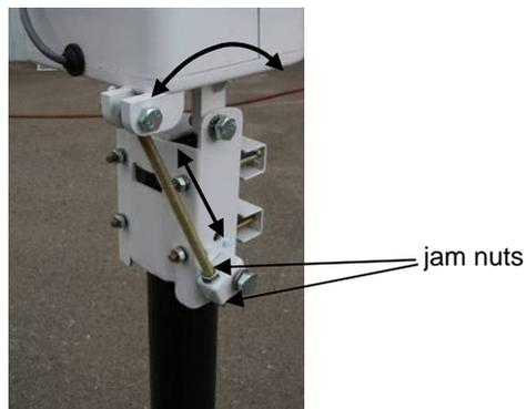
5. Adjust the roll by loosening or tightening the turnbuckle after loosening the main clamp bolts.
