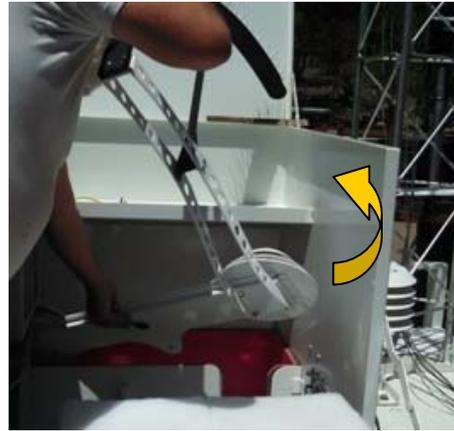
Mount T-tail to top of Tail Mast and plug in the two instruments to the nearest connectors. These connectors have a locking ring that must be lightly twisted until the plug seats fully then locked with a 180-degree clockwise turn.
