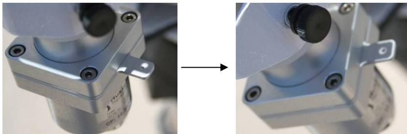
3. Gently tighten the mounting screws to hold the instrument firmly. Be careful to preserve your alignment while tightening the screws.
