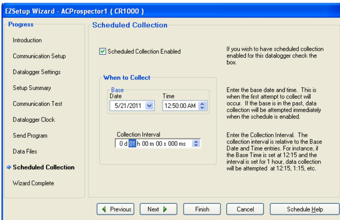
The scheduled collection interval and ‘first download’ base time are selected here. Clicking next will allow the specification of retry intervals if the first attempt is not successful. There are two stages of ‘retries’ designated ‘Primary’ and ‘Secondary’ each of which can have a different interval.
