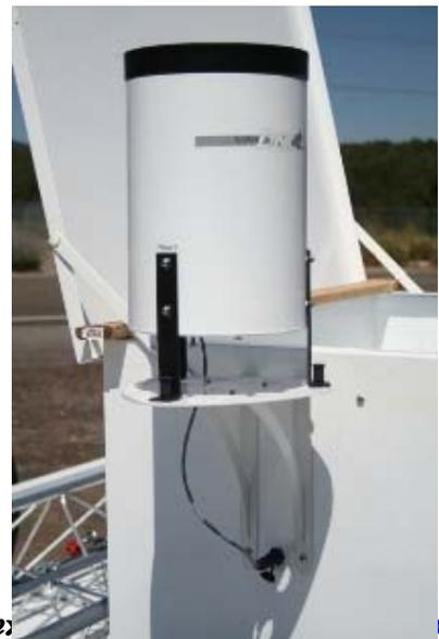
Remove the dust cap from the small receptacle beneath the mounting plate and attach the rain bucket signal cable.
