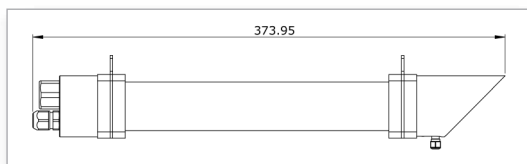
◀ Figure 1: DR01 Pyrheliometer mechanical dimensions
