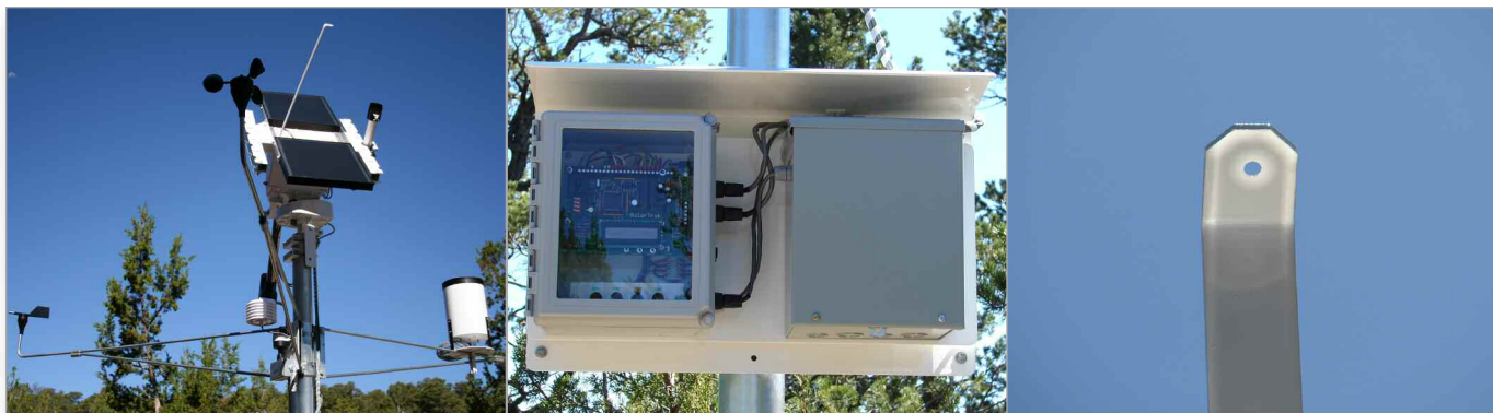
▲ Figure 1: PST Prospector™ system with MiniTrak™ and fully integrated turnkey weather monitoring station
